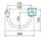
Watertight: to ensure the watertight of the channels, it is advisable to use a bituminous sealing adhesive. As a complete and long lasting guarantee of the absence of leakages through the joints of the channels, it is possible to heat-weld the joints.
